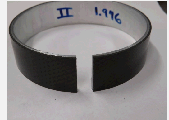
Carbon Fiber - 45° skew, 4 plies
