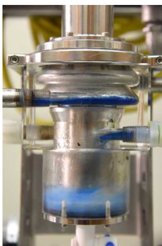
Fig. 4. Operating 5-cm centrifugal contactor with plastic housing.
