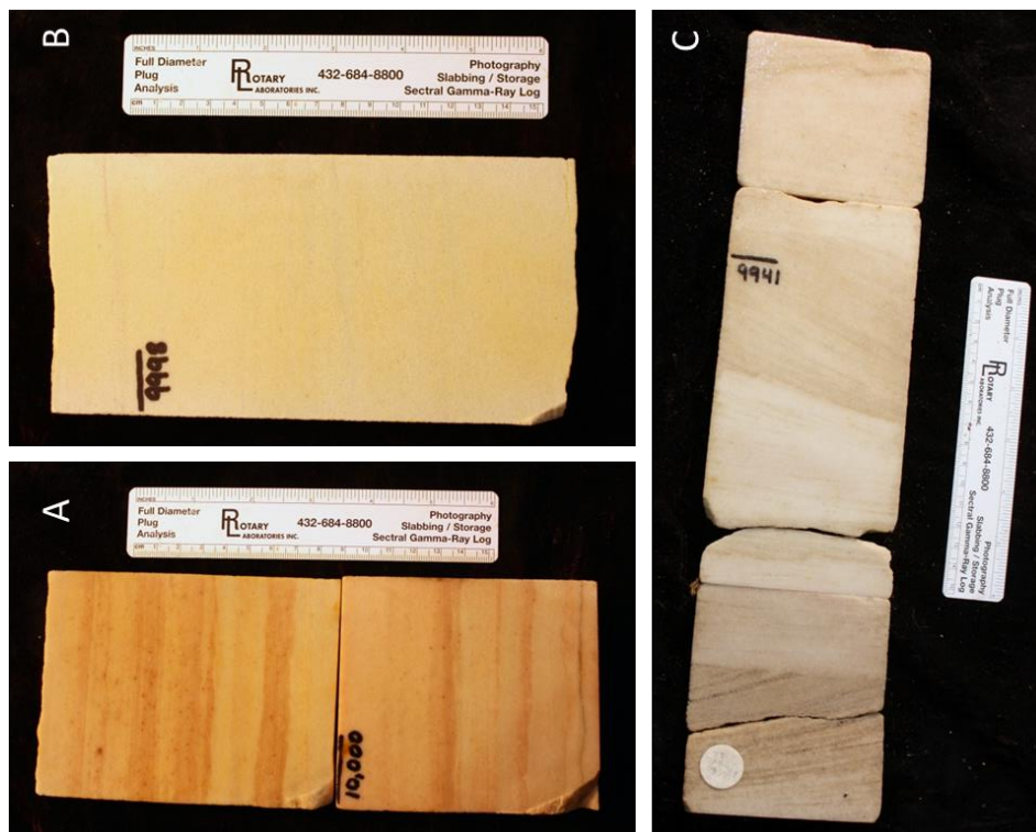
Figure 2-5. Whole core photographs of Lithofacies 1 showing fine to medium-grained planar laminated sandstone (A), massive fine-grained sandstone (B), and coarse-grained cross-bedded sandstone (C).
