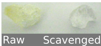
Figure 9 – Picture of a single crystal of BaBrCl grown in a standard Bridgman furnace (left) and one grown after a scavenger procedure (right). The yellow color is due to the presence of color centers/defects created during the growth process. The scavenger process allows for a mitigation of the defects and so an improvement of the material performance.
