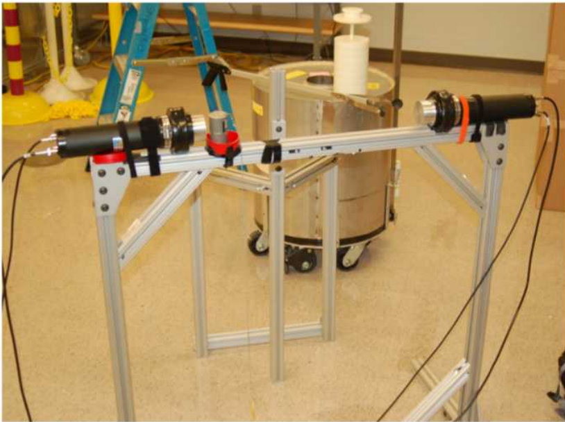
Fig. 1. Setup of the two detectors with Am-Be source in position.
