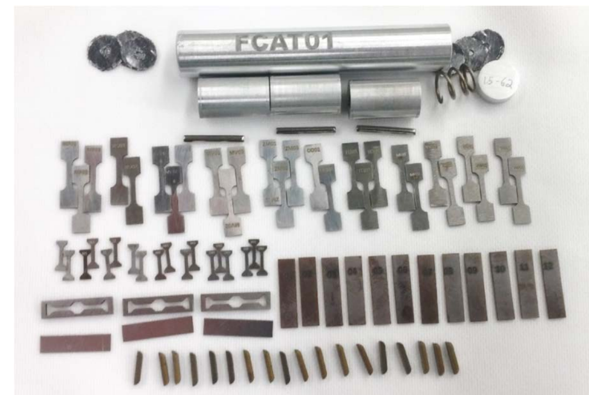
Figure 1: Image of disassembled irradiation capsule designed for exposure of specimens in HFIR.
