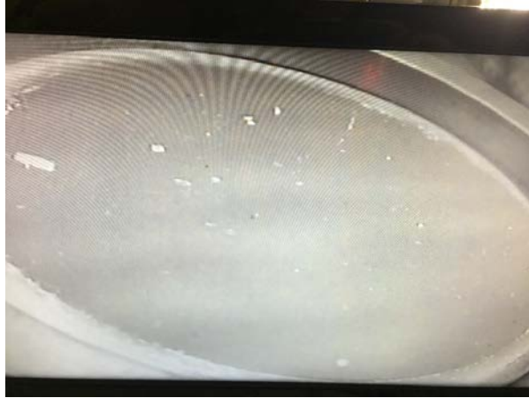
Figure 3.12. Solids on Filter after DEF Filtration
