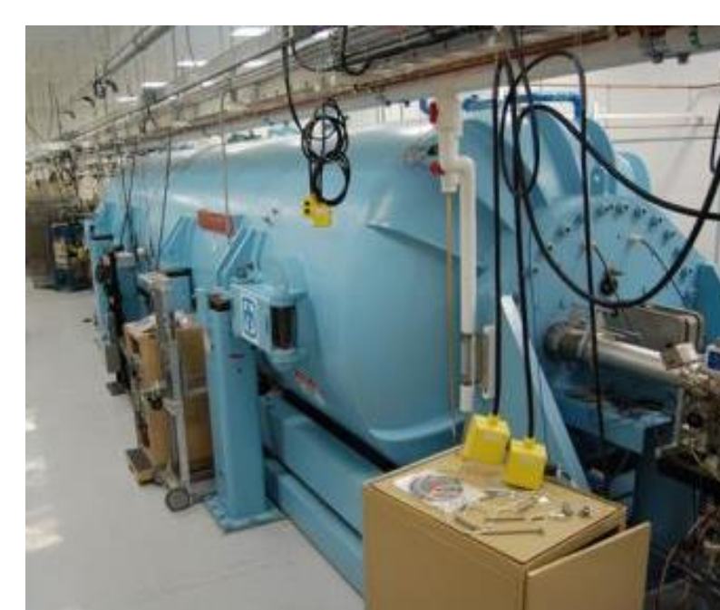
6 MV Tandem Heavy Ion (e.g. Au) beams
