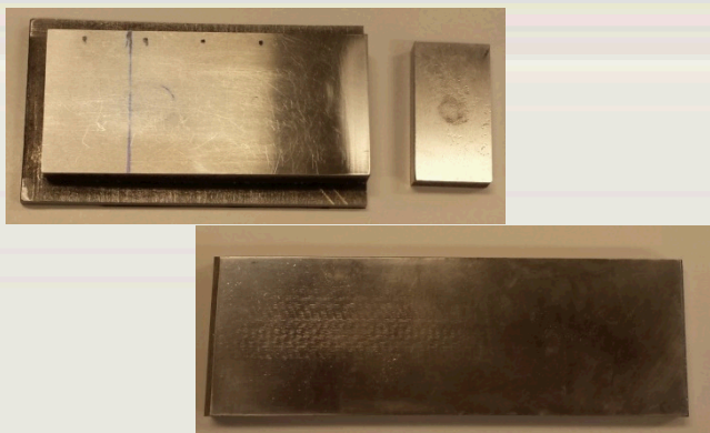
LENS 304L (top) & wrought 304L (bottom) samples
