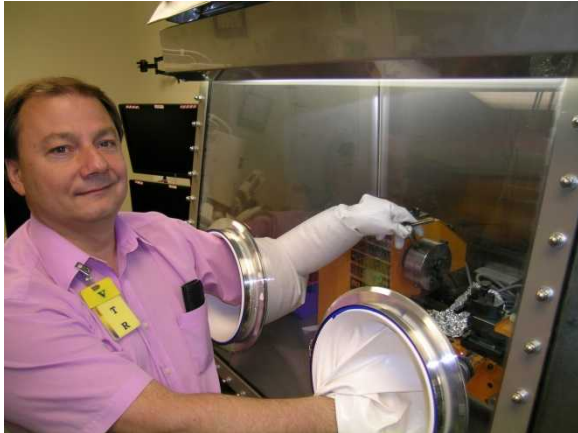
Glove box Lathe is used to cut through the large flange.
