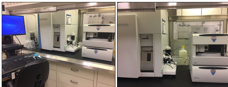
Fig. 2 Photo of the coupled HPIC-ICPMS system in a radiological fume hood
