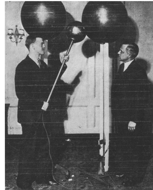
Robert J. Van de Graaff demonstrating his 1.5 MV electrostatic generator to Karl T. Compton in 1931. (from D. Allen Bromley, Nucl. Instr. Method. 122, 1-34 (1974))
