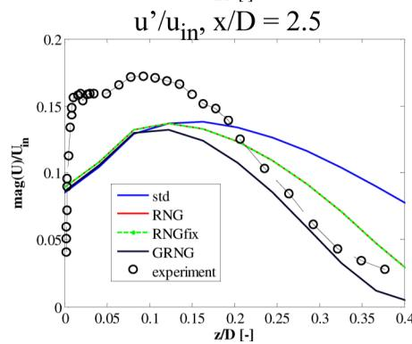
The RNG and GRNG models both perform reasonably well for all simulated diesel engine-like flow conditions
