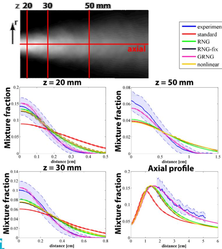
The GRNG model yields the most accurate flame structure predictions
