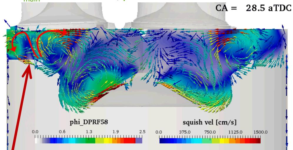
The upper portion of the jet impinges on the head and splits. The outward bound portion is redirected downward at the liner. The upper toroidal vortex transports the remaining mixture inward, away from the mixture in the outer squish region.
