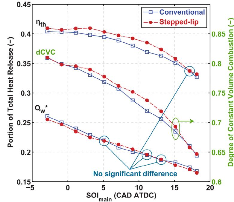
Thermal efficiency gains with the stepped-lip piston are greatest for main injection timings between 3 and 13 CAD ATDC
