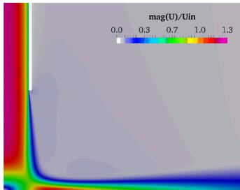
The GRNG turbulence model provides the most accurate velocity-profile predictions and reasonable predictions of velocity fluctuations near the jet.
