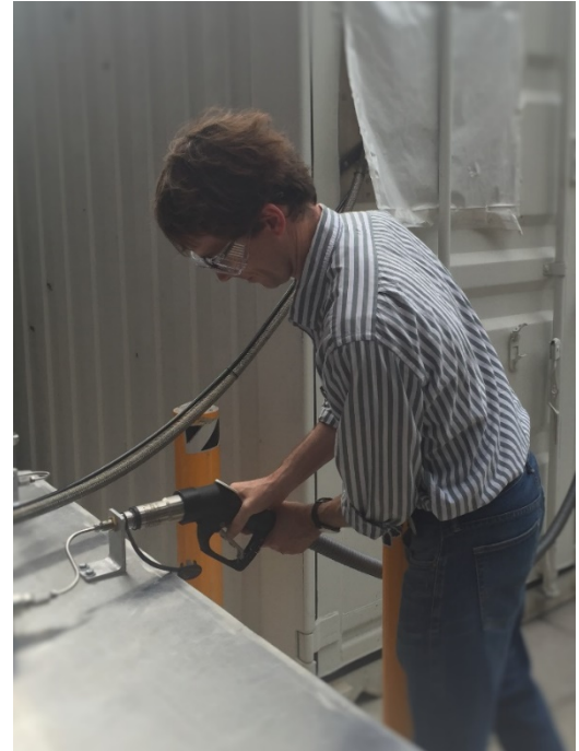
SIMPLEFUEL TEAM MEMBER CHRIS O'BRIEN IS CONDUCTING A TEST FUELING IN PREPARATION OF THE DEMONSTRATION PHASE
