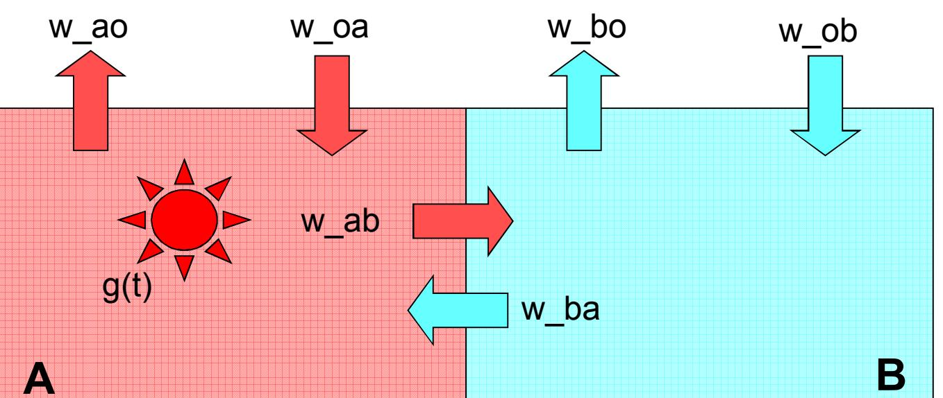
The two-compartment model is parameterized with the volumes of each compartment, the airflow rates between the compartments and the time varying source located in room A.
