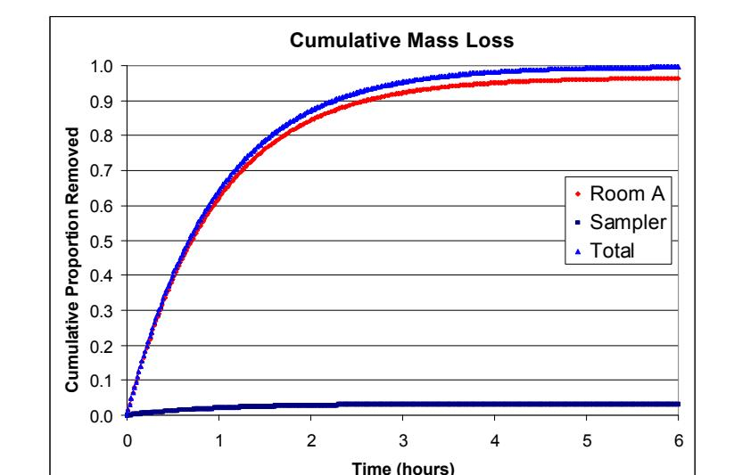
Parameters for these calculations include room volumes of 150 and  $0.1\text{m}^3$  for room A and the sampler,  $w_{oa} = w_{ao} = 150\text{m}^3/\text{hr}$ ,  $w_{ab} = w_{ba} = 10\text{m}^3/\text{hr}$ , sampling efficiency = 0.50. The fraction of the initial mass extracted by the filter at 12 hours is 0.032
