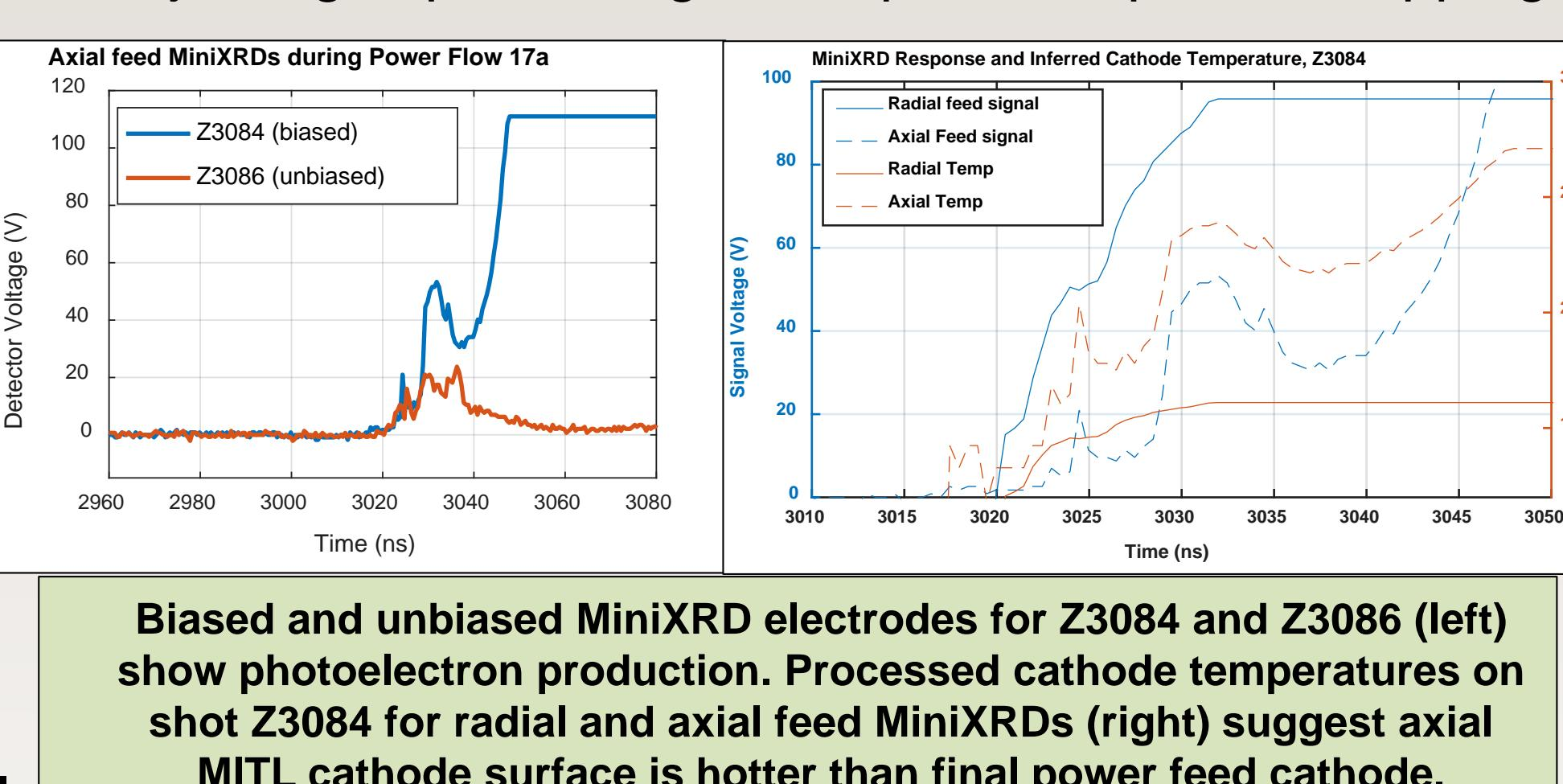
Biased and unbiased MiniXRD electrodes for Z3084 and Z3086 (left) show photoelectron production. Processed cathode temperatures on shot Z3084 for radial and axial feed MiniXRDs (right) suggest axial MITL cathode surface is hotter than final power feed cathode.
