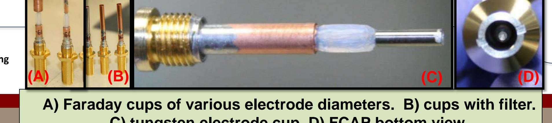
A) Faraday cups of various electrode diameters. B) cups with filter. C) tungsten electrode cup. D) FCAP bottom view.
