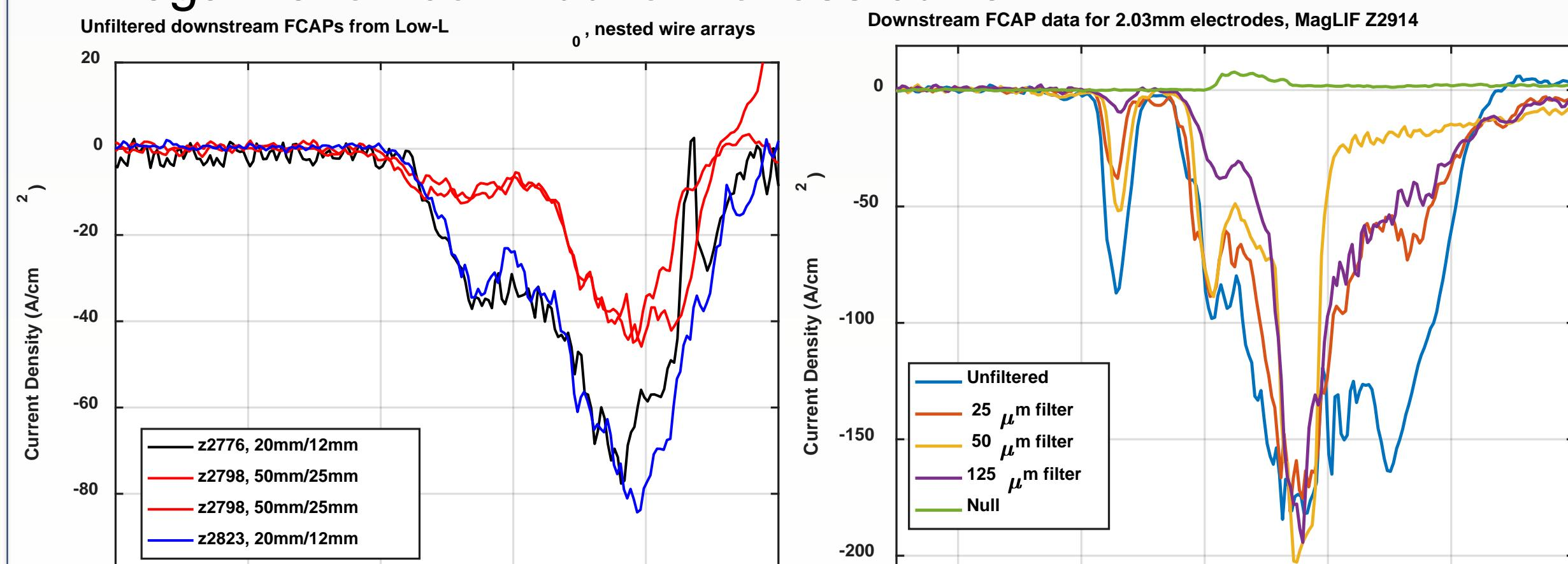
Unfiltered downstream FCAPs show repeatable convolute behavior for low- $L_0$  wire arrays (left). High- $L_0$  MagLIF loads (right) present higher current densities; varying filter responses suggest either convolute asymmetry or significant low-energy electrons.
