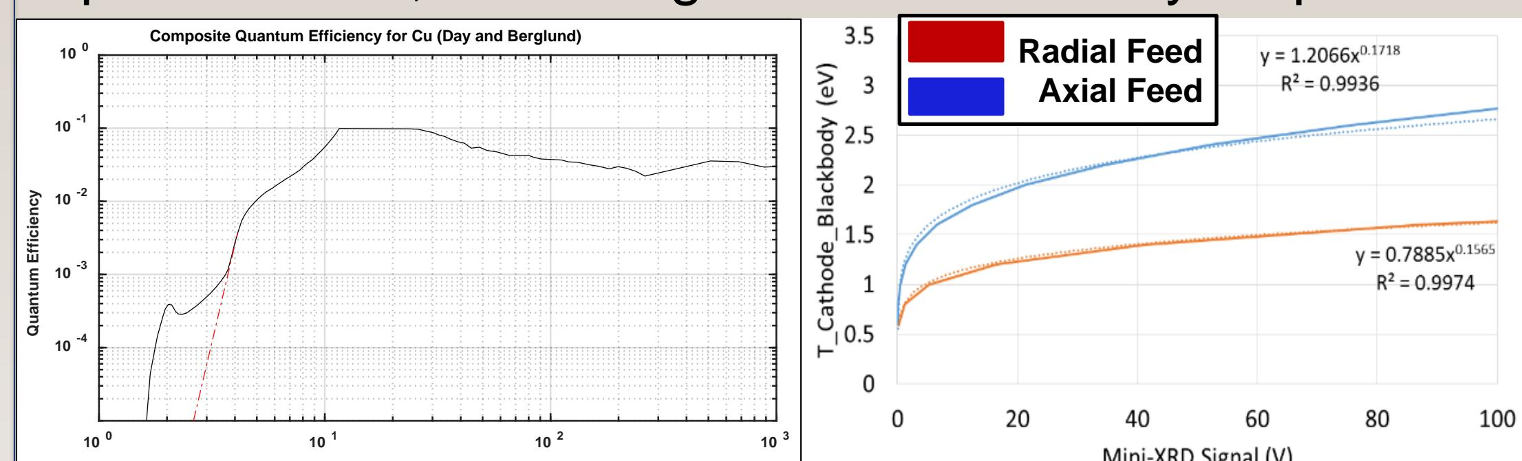
Computed blackbody spectral intensity, with geometric effects, is convolved with copper photoelectron quantum efficiency (left, from Day<sup>2</sup> and Berglund<sup>3</sup>) to determine detector current. MiniXRD voltage measurements scale to effective observed blackbody temperature (right).
