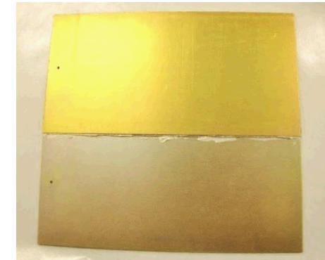
Preparation of samples (a) overlap shear samples being prepared using Loctite Ablestik 2902, (b) cured overlap shear panel which will be cut to obtain 5 lap shear samples that will be aged at elevated or room temperature.
