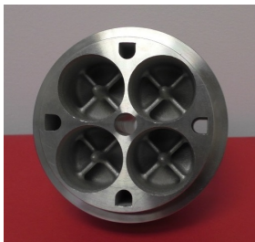
Figure 15. 3D printed stainless steel swirl bubbler.
