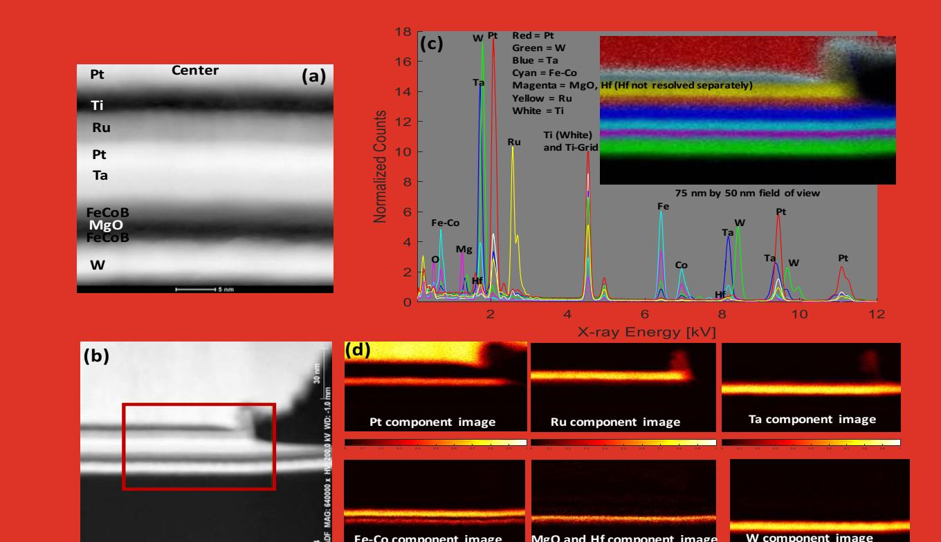
**Conclusion: FIB/STEM/EDS analysis of morphology, structure, chemical constituents can provide insight into variation in properties among specific devices and guide changes in fabrication and processing**
