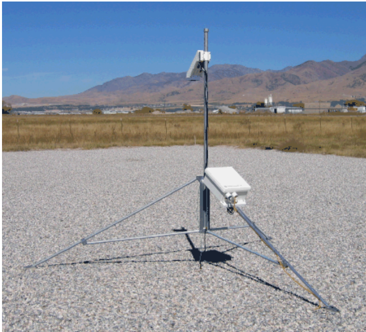
Tripod-mounted electric field mill, CS110 Electric Field Meter , Rev. 4/12, p. 15
