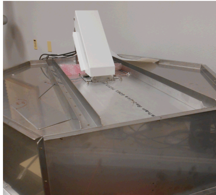
Electric field mill mounted in parallel plate test structure
