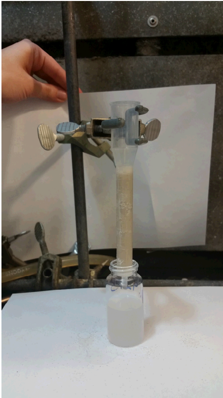
Column testing in sand
