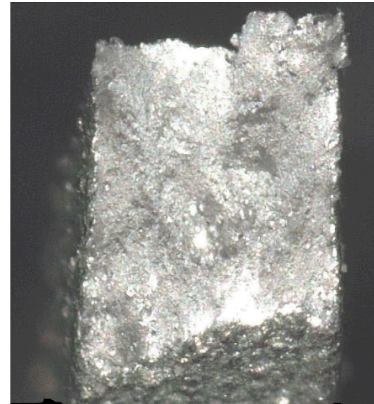
B2, fracture surface optical image by structured light scanning
