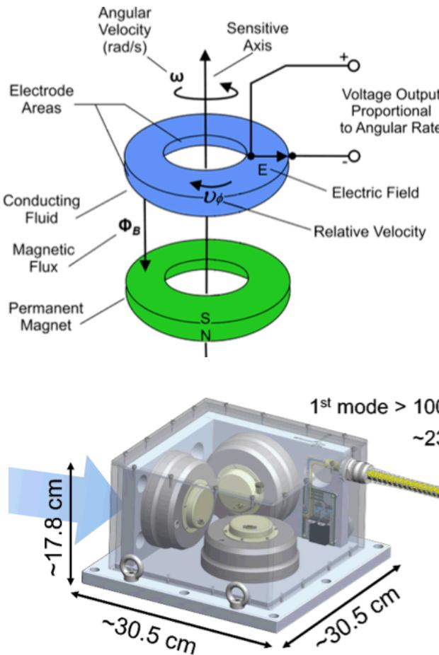
A conductive fluid acts as a proof mass. Seismic motion rotates a permanent magnet fixed to the sensor case relative to the fluid, creating an electrical signal proportional to angular rate.
