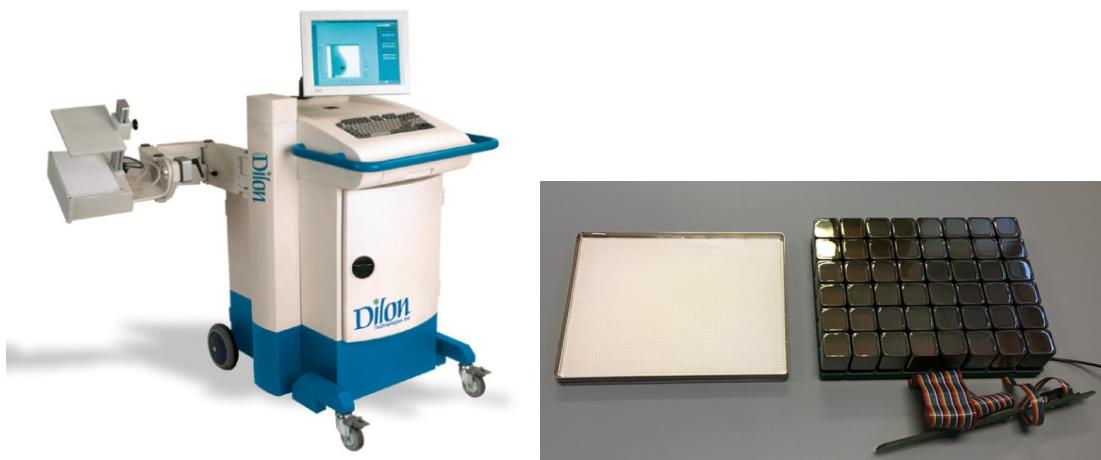
Figure 2: (Left) Dilon 6800 Gamma Camera based PSPMTs. (Right) NaI(Tl) crystal scintillator array next to PMPMT based detector module.
