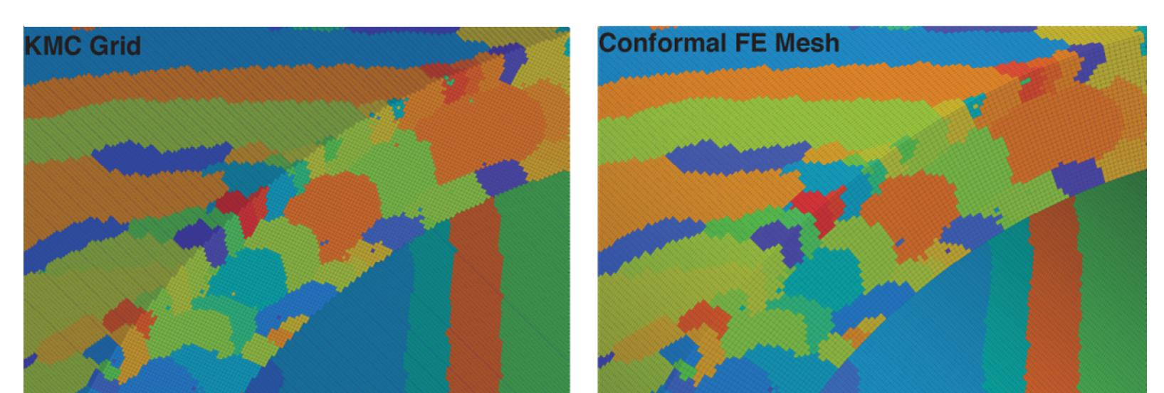
Voxelized Monte Carlo microstructures were remeshed to a conformal finite element mesh of ~ 55,000,000 elements.
