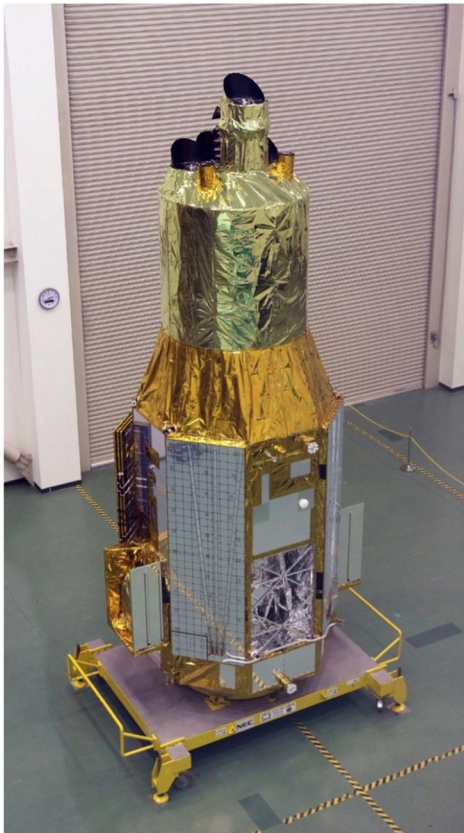
Fig. 1 A photograph of the Hitomi satellite. The height in this launch configuration is 7.86 m.
