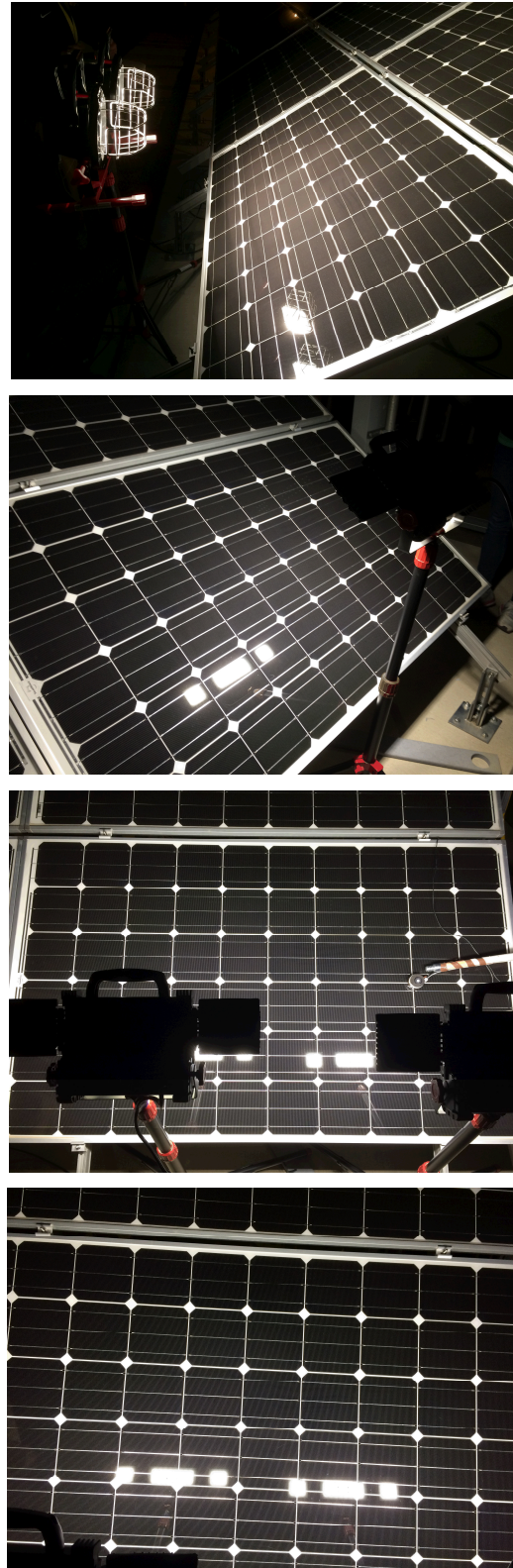
Fig. 7. Photos of the test setup: (a) two 1200W halogen lights; (b) one 2500 Lumens LED light; (c) two 2500Lumens LED lights; (d) top view of illumination by two LED lights, showing significant non-uniformity of the illumination
