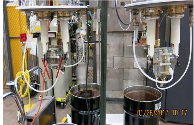
Figure 3. The switches are mounted through the cable guides on the top tank leads.
