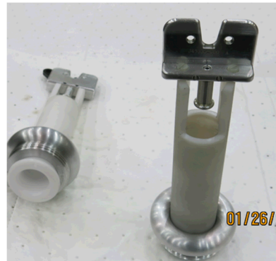
Figure 4. An early cable guide. The switch is mounted at the top metal plate.
