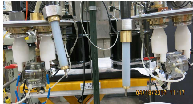
Figure 9. The switches are suspended with the new successful cable guides. The cables are outside of the guides. The oversize banana plugs are also visible.
