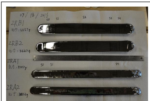
Fig. 1: Production of the zone-refined ingots per run with two stages and a total of 14 passes. Two ingots below the ruler are from the first stage and two ingots above the ruler are from the second stage. The net impurity levels are 6.0 \times 10^{10}/\text{cm}^3 , 7.7 \times 10^{10}/\text{cm}^3 , and 9.1 \times 10^{10}/\text{cm}^3 , for S1, S2, and S3, respectively.
