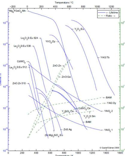
Figure 1. The lifetime and intensity ratio of several thermographic phosphors as a function of temperature [1].
