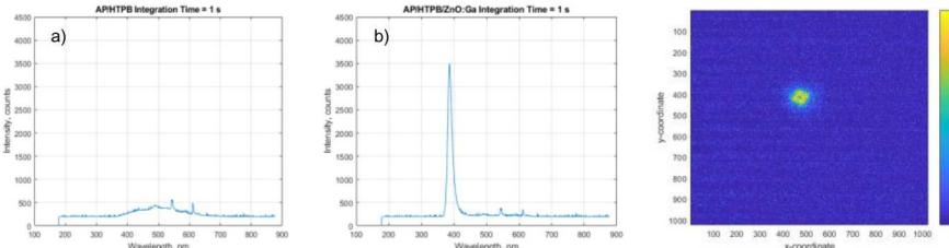
Figure 2. Plots comparing the spectra of the induced emission from an AP/HTPB solid propellant a) without and b) with ZnO:Ga phosphors added as inclusions. A peak near 390 nm is expected for this phosphor at room temperature.
