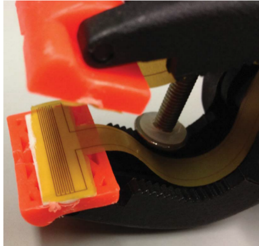
Figure 54. Photograph of interdigital capacitive sensor described elsewhere [1]. The sensor accommodates wires with diameter up to approximately 3 mm. Number of electrode digits: N = 14 , width of each digit: w = 0.1 mm, separation between each digit: g = 0.3 mm, and digit length: l = 25 mm.
