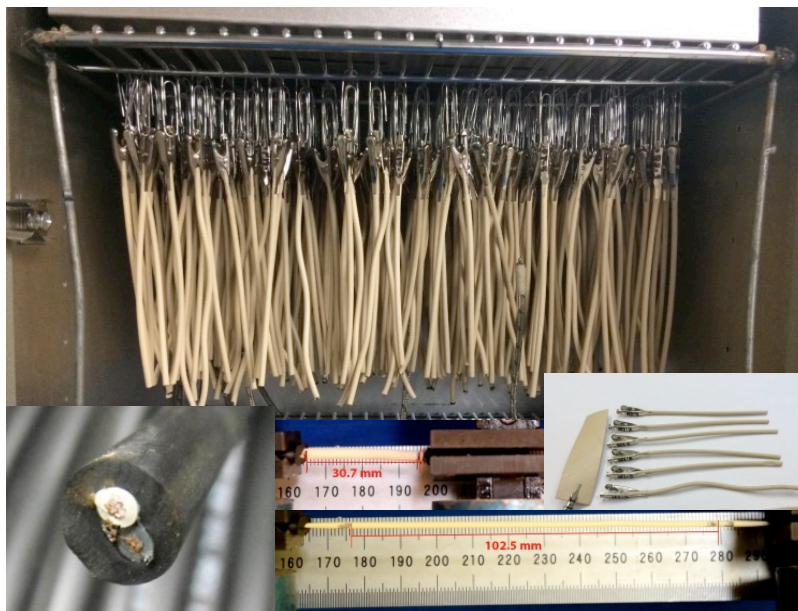
Figure 5. Low voltage cross-linked polyethylene (XLPE) insulated cable (lower left). XLPE insulation samples in oven rack (above). Example XLPE sample set (right). Image analysis of tensile performance (lower center).
