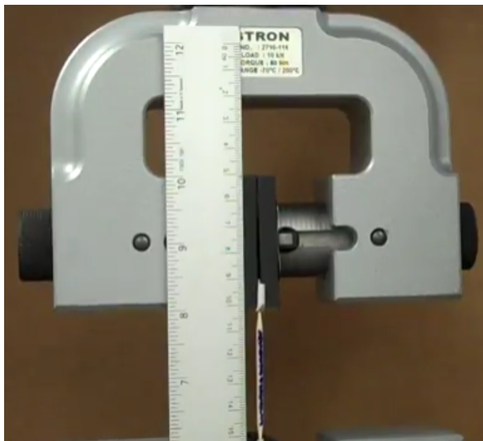
Figure 23. Equipment set-up for measuring elongation-at-break on aged XLPE samples.
