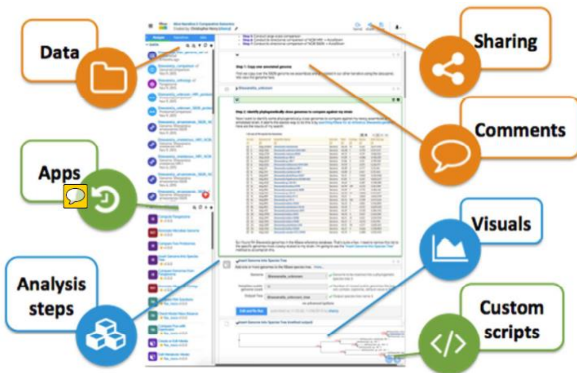
Figure 7. Overview of a KBase Narrative. A Narrative is a shareable, reproducible computational experiment that can include data, analysis steps, results, visualizations, and commentary.
