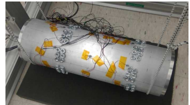
Masses bonded at anti-nodes
