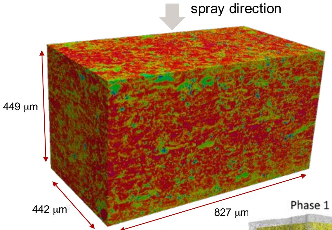
Ta (1) and Ta-oxide (2) phases are distinguished from pores.
