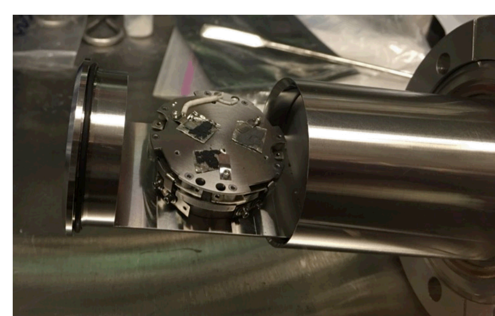
XPS Clean Transfer Holder Compatible with both Sandia and ALS XPS systems
