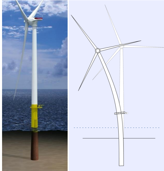
Figure 4 – GE Haliade150-6MW wind turbine on a Monopile and 1st bending Side-to-Side mode in a Monopile fixed-bottom substructure 5
