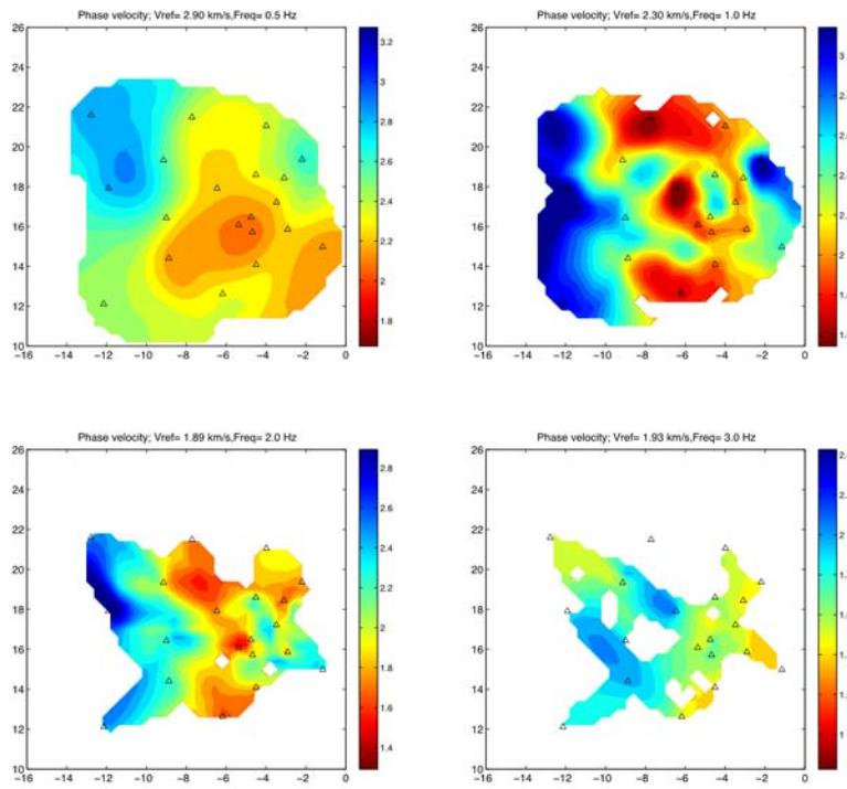
Figure 8. Phase velocity maps at four different frequencies plotted where resolution is greater than 0.
