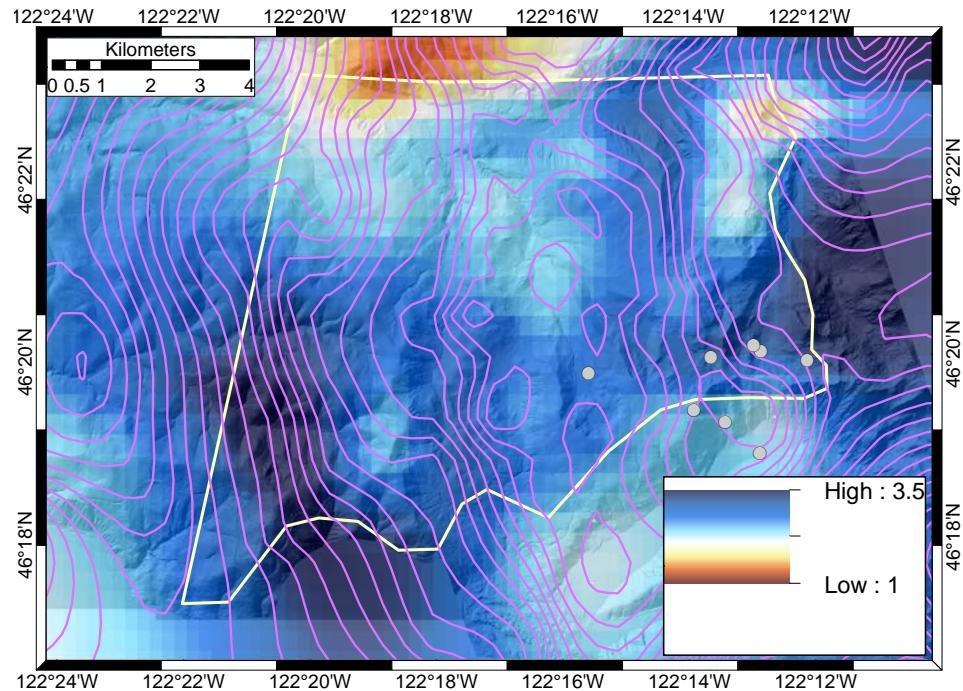
Figure 8: Resistivity depth slice at 1500 m with isostatic gravity contours (magenta lines) and earthquake locations (gray circles) within 500 m of the depth slice.
