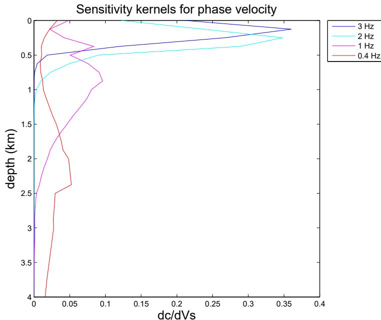
Figure 7. Sensitivity kernel for each of the frequencies used. Shows how deep the structure of the phase velocity is sensitive to.
