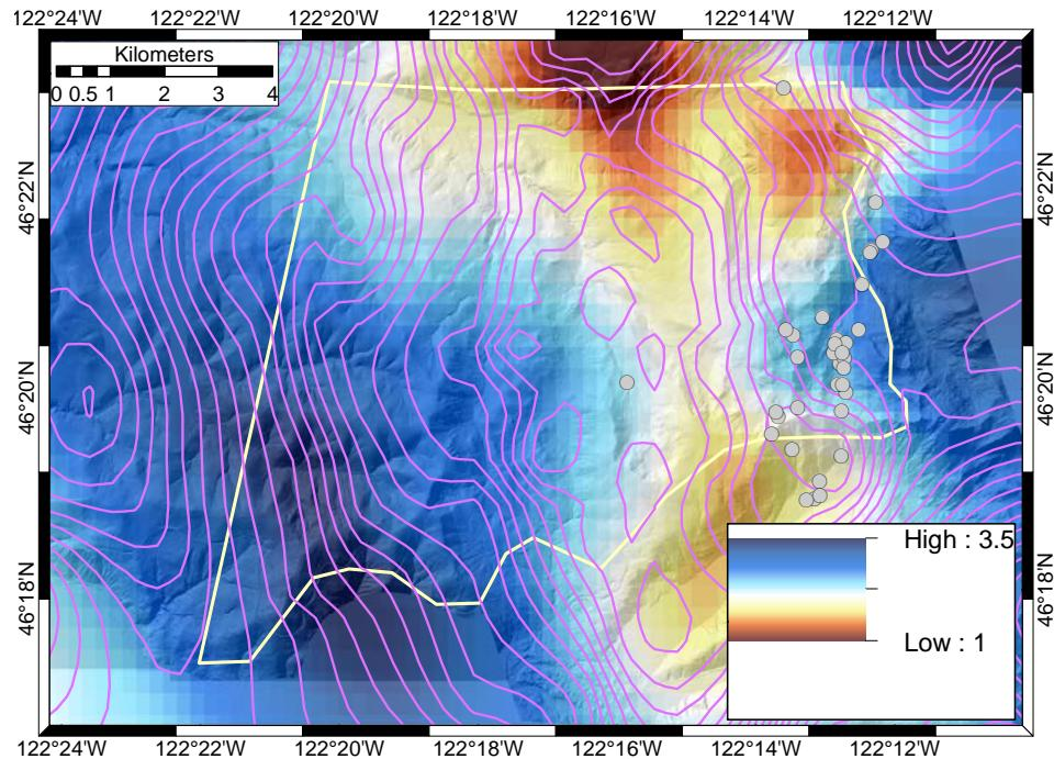
Figure 10: Resistivity depth slice at 3260 m with isostatic gravity contours (magenta lines) and earthquake locations (gray circles) within 1000 m of the depth slice.
