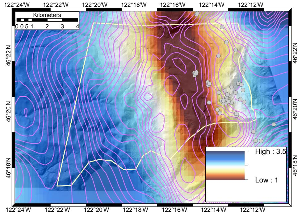
Figure 11: Resistivity depth slice at 5860 m with isostatic gravity contours (magenta lines) and earthquake locations (gray circles) within 1000 m of the depth slice.
