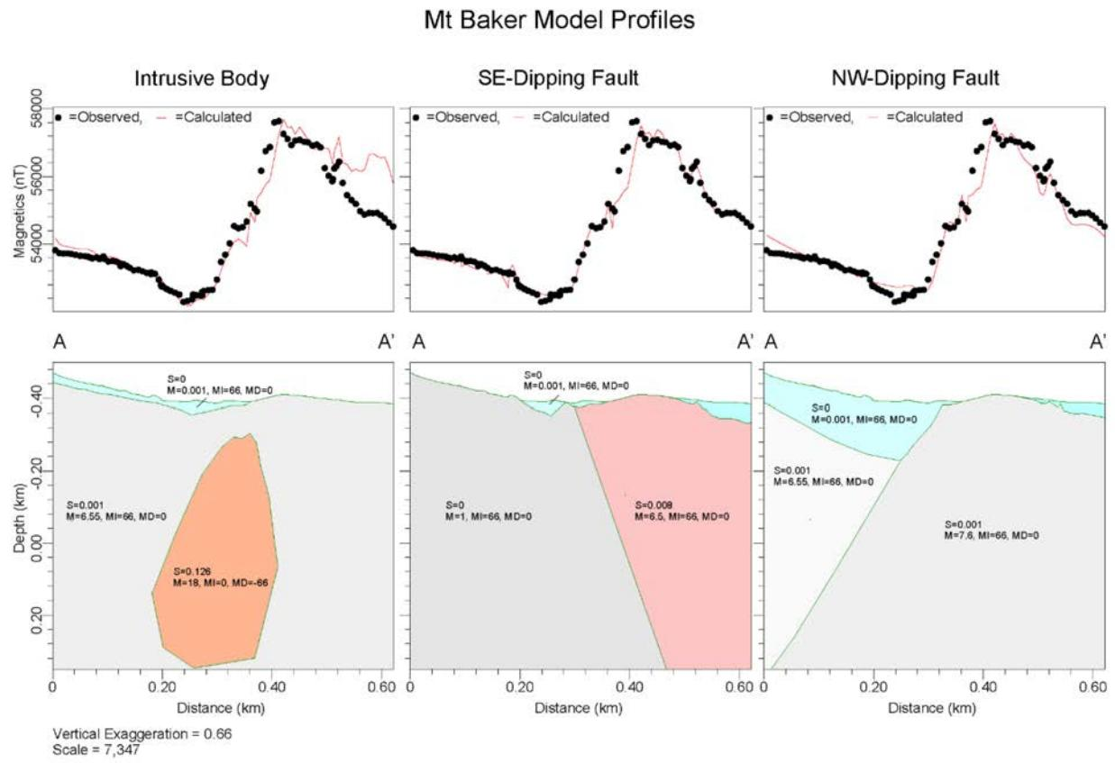
Figure 20. Three different 2D Potential field models along profile AA' in the Mount Baker study area. Top panels show observed (black circles) and model (red line) magnetic anomalies. Lower panels display potential field models with individual model bodies colored by rock unit. Profile location shown on Figures 4 and 7.
