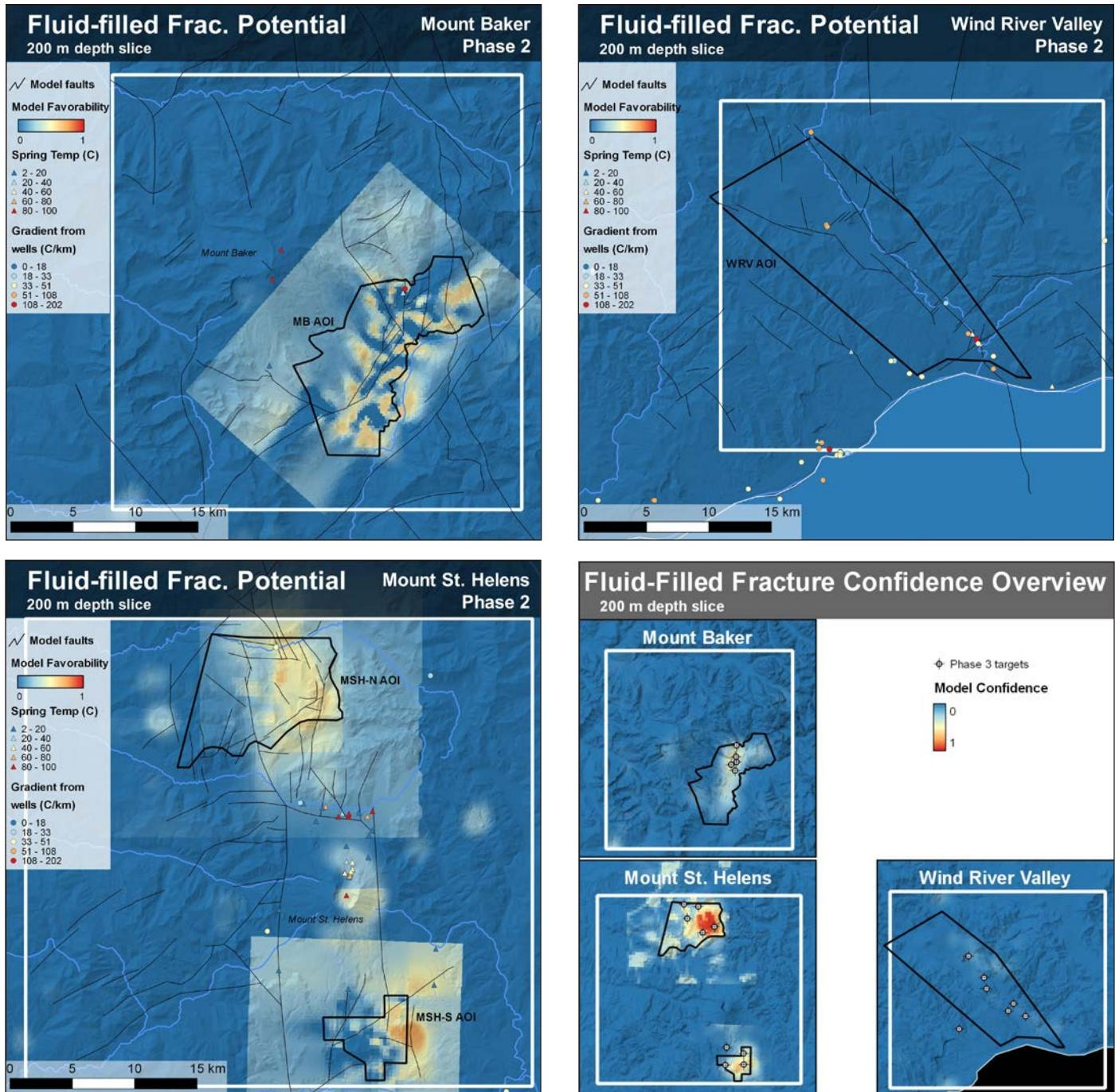
**Figure 5.** Phase 2 fluid-filled fracture potential at 200 m depth and overview of confidence. Data sets vary substantially between study areas and make comparisons between areas difficult. Potential models at 2 km depth are provided in Appendix I and confidence models are provided in Appendix J.
