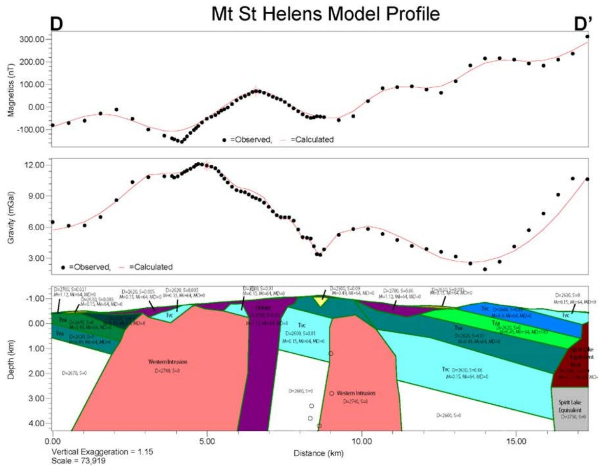
Figure 24. 2D Potential field model along profile DD' in the Mount St. Helens study area. Panels show observed (black circles) and model (red line) anomalies for magnetic (top) and gravity (middle) fields, and potential field model with individual model bodies colored by rock unit (bottom). Open circles are earthquake hypocenters from the PNSN catalog. Profile location shown on Figure 8.
