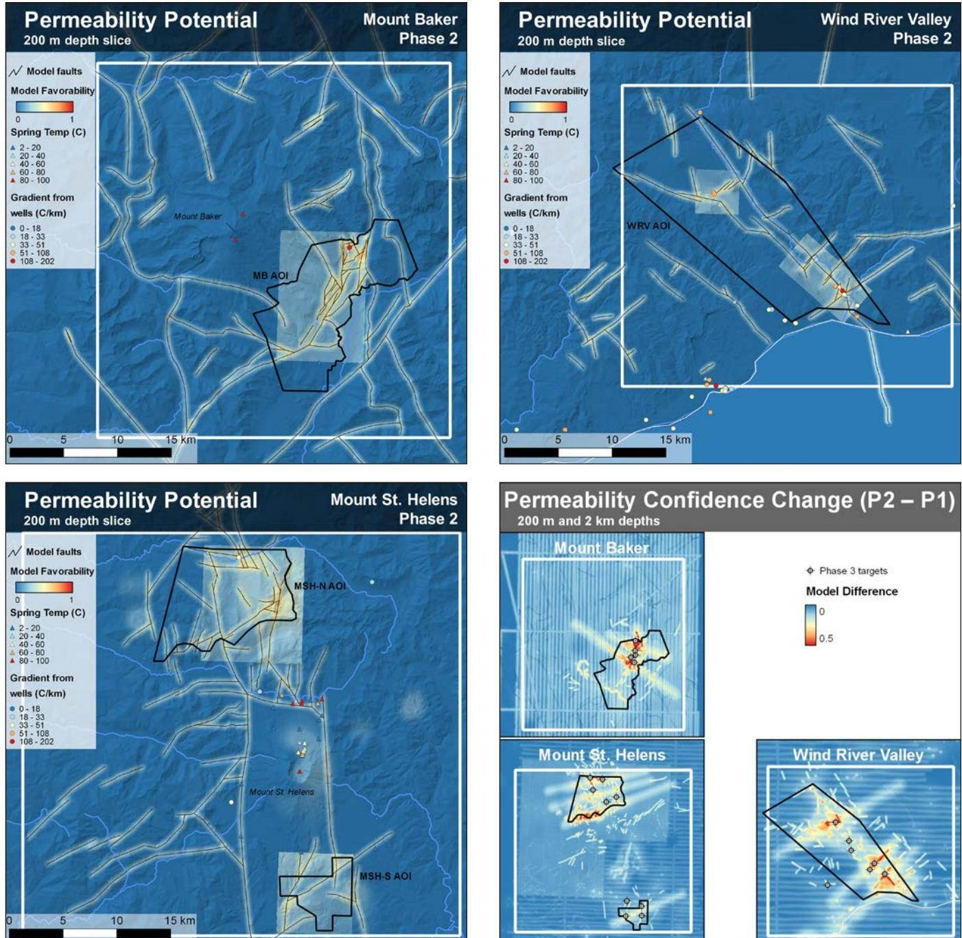
**Figure 4.** Phase 2 permeability potential at 200 m depth and change in confidence from Phase 1. Confidence increases are the result of new mapping, lidar interpretation, the inclusion of new gravity and magnetic data, modeled cross sections, and updated and refined geomechanical models, and opportunistic data collection near WRV. Potential models at 2 km depth are provided in Appendix I and confidence models are provided in Appendix J.
