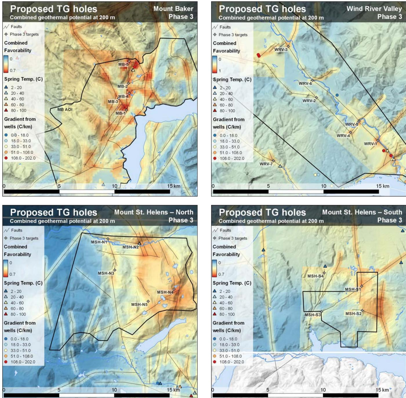
**Figure 12.** Proposed temperature-gradient holes (TGH) at the Mount Baker (upper left), Wind River Valley (upper right) and Mount St. Helens northern and southern AOIs (bottom). Maps show major faults at 200 m depth and favorability values from the combined geothermal model. Values are scaled to 0.7 which is the maximum value achieved in any of the three study areas.
