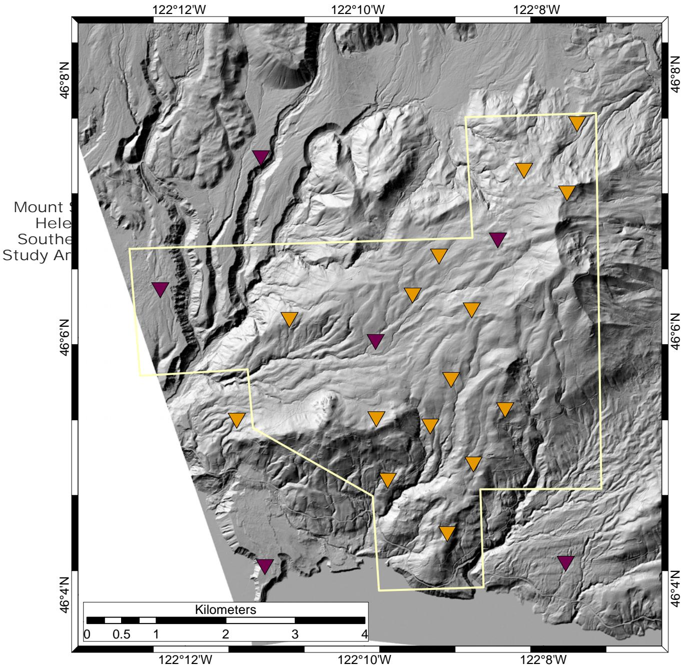
Figure 1: Area of interest south of Mount St. Helens (yellow line), location of MT stations collected for this survey (orange triangles), and existing MT stations.
