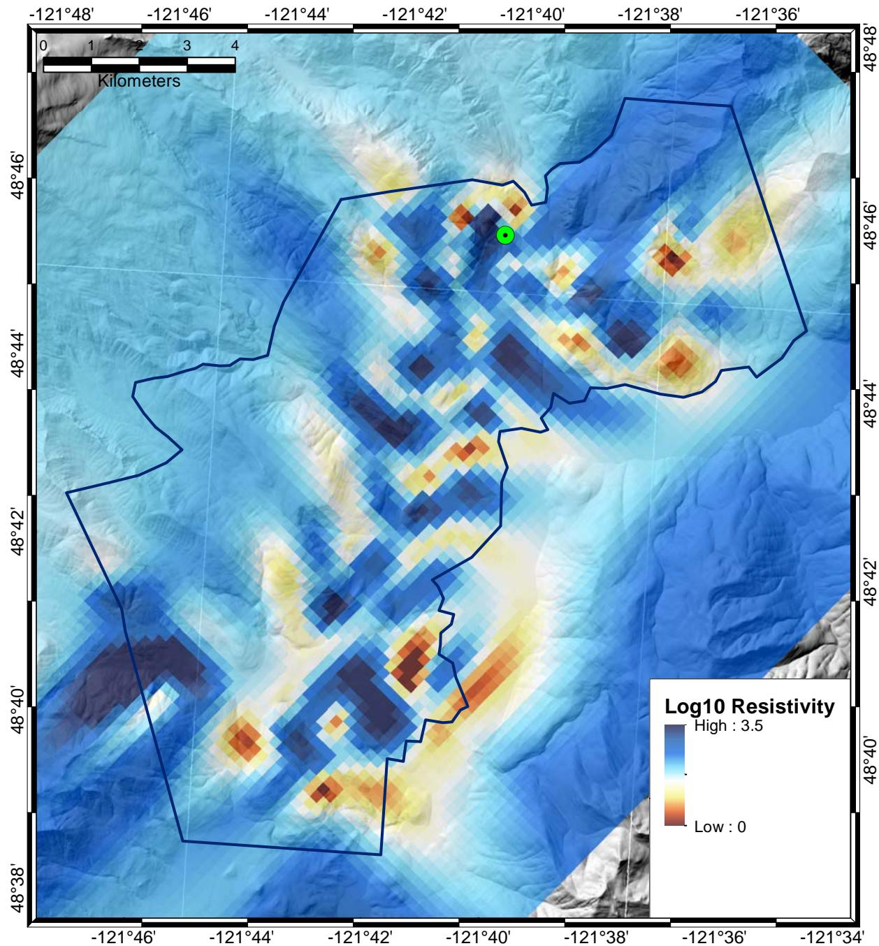
Figure 4: Depth slice at 290 m. Green dot is hot spring location.
