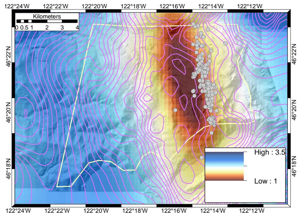
Figure 12: Resistivity depth slice at 7860 m with isostatic gravity contours (magenta lines) and earthquake locations (gray circles) within 1000 m of the depth slice.
