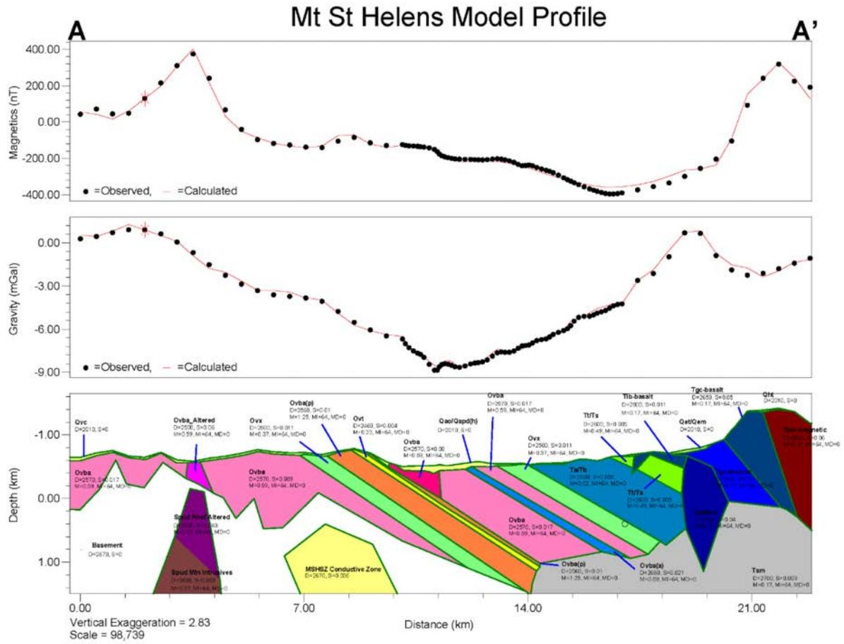
Figure 21. 2D Potential field model along profile AA' in the Mount St. Helens study area. Panels show observed (black circles) and model (red line) anomalies for magnetic (top) and gravity (middle) fields, and potential field model with individual model bodies colored by rock unit (bottom). Open circles are earthquake hypocenters from the PNSN catalog. Profile location shown on Figure 8.
