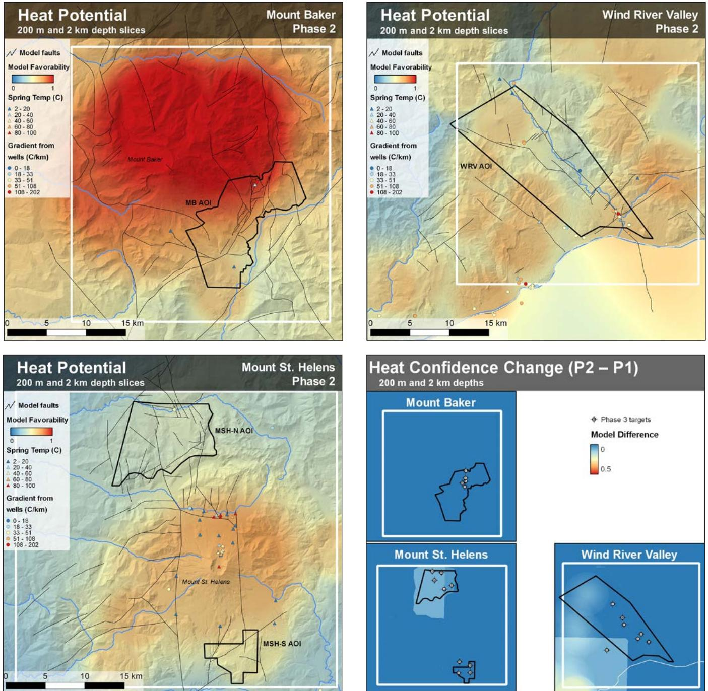
**Figure 3.** Phase 2 heat potential and change in confidence from Phase 1. Confidence increases are largely the result of new mapping at MSH, and opportunistic data collection near WRV. Individual confidence models are provided in Appendix J.
