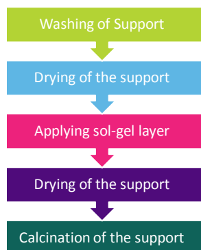
Figure A-C. 2. Steps involved in the pre-treatment of the PSS support.
