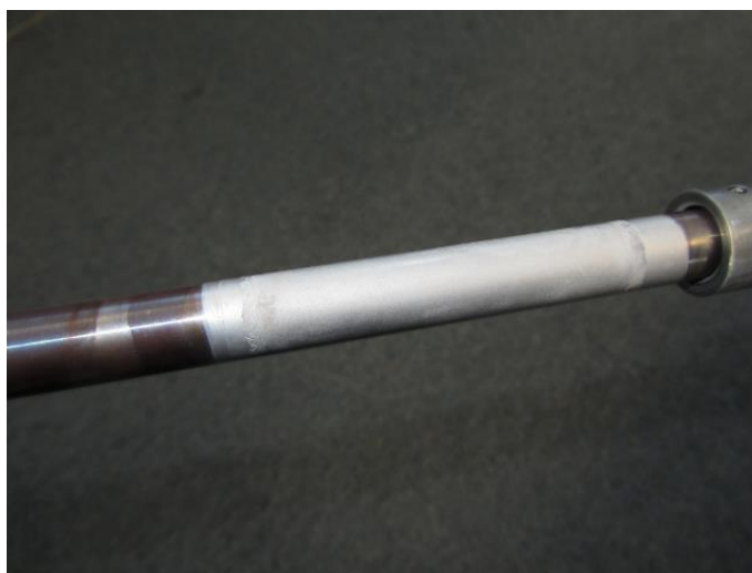
Figure 10. 6. Seven \mu\text{m} thick supported palladium membrane (X101) with \sim 20 \text{ cm}^2 surface area on top of a high temperature barrier layer and Hastelloy porous support.
