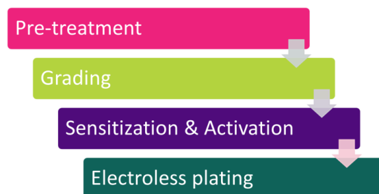
Figure A-C. 1. Main processes involved in WPI synthesis of pure Pd membranes.
