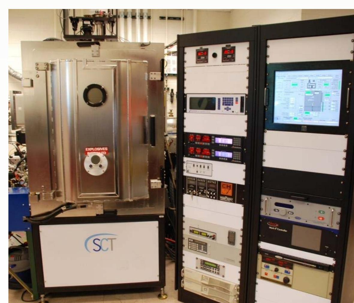
High Vacuum Chamber for Performing PVD (left), Schematic of PVD process (center), and Model of Deposition Fixture (right).
