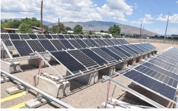
Fig. 5. Bifacial PV module test bed at Sandia. Four rows of PV modules with tilt angles from 15^\circ to 45^\circ . Backside irradiance measured for top and bottom of PV module near the center of each row. Front side irradiances are also measured.
