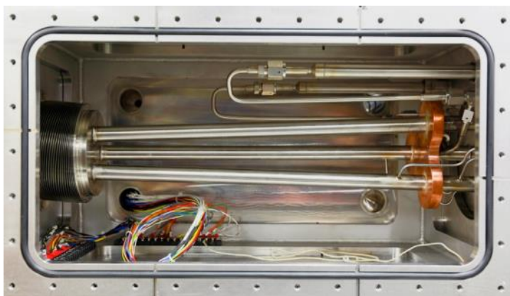
Fig. 1 A 3-barrel shattered pellet injector prototype installation in a guard vacuum chamber [5].
