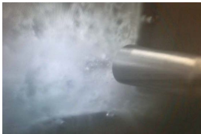
Fig. 2 Shattered pellet spray from a 25mm neon deuterium mixture pellet in a 65degree miter bend shatter tube. The spray results in mostly gas with significant backward reflected spray
