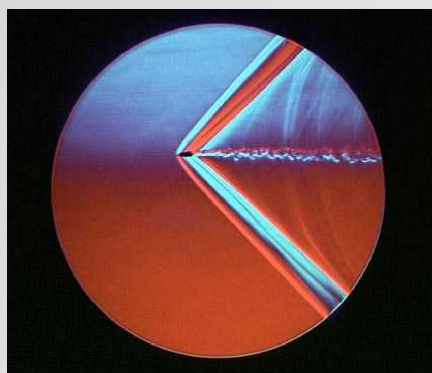
Schlieren high speed projectile image
