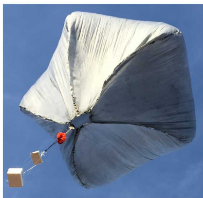
Figure 1: A Heliotrope just after launch, showing the darkened envelope, open bottom, scientific payload and tracker packages (white boxes), and parachute (orange).
