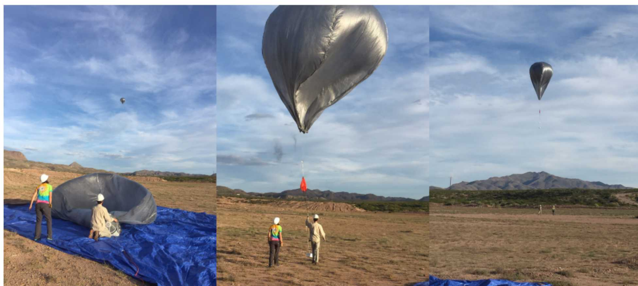
Figure 2: Solar hot air balloons carrying infrasound sensors launched as part of the 2017 Heliotrope experiment.
