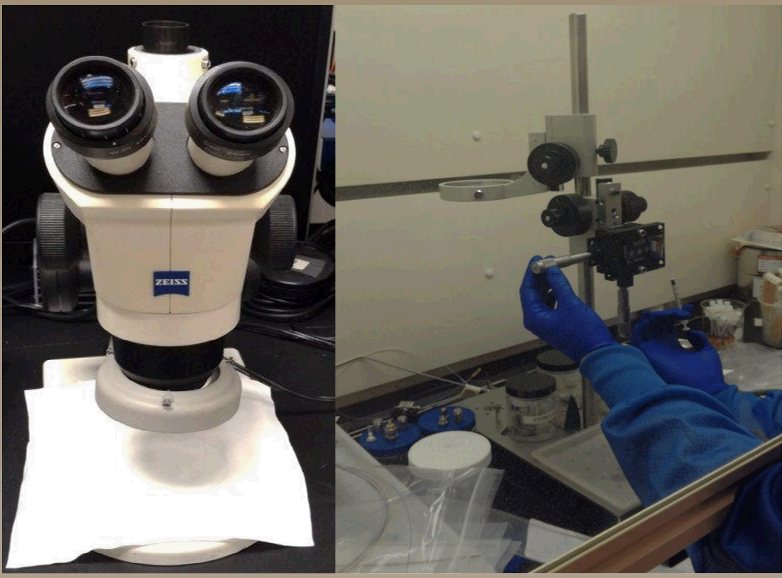
Figure 3: A microscope and multi-meter were used to ensure the electrodes were in the correct position for a mercury drop size of .3mm to .6mm.
