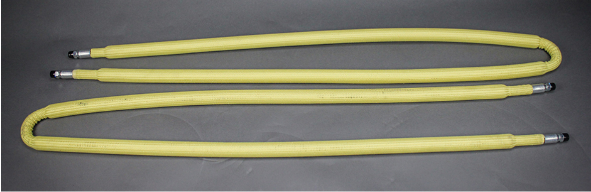
Figure 11. Complete conformable pressure vessel ready for pressure and permeability testing.
