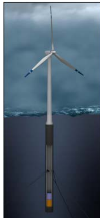
Figure 93. a) WindFloat Semi-Submersible (31) and b) Hywind Spar (32).
