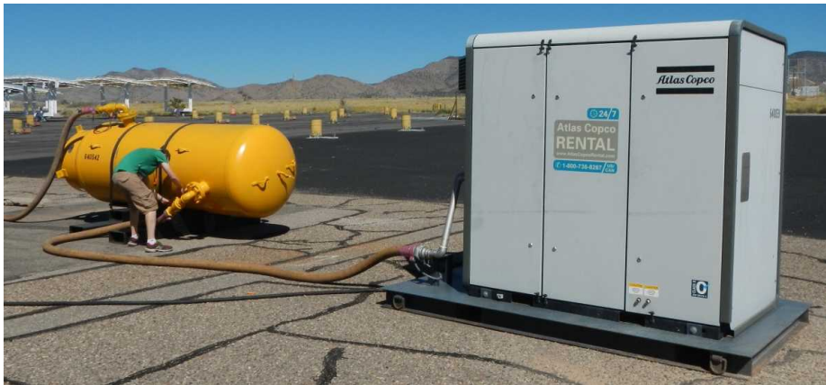
Air compressor and 1000 gallon air receiver tank
