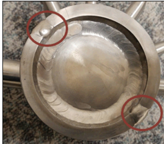
Full penetration seam weld
