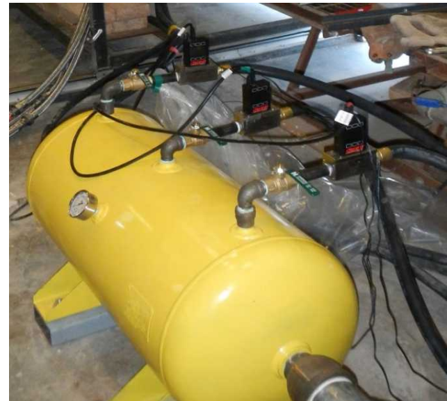
Alicat mass flow rate sensors attached to the three outlet manifold tank
