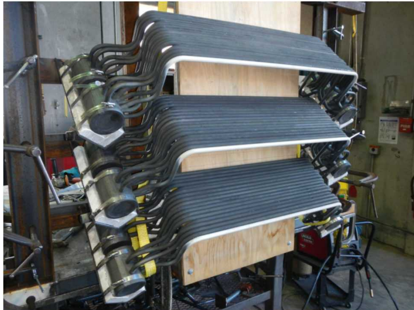
Bladed receiver panels with front tube painted white with VHT Flame Proof Header Paint.
