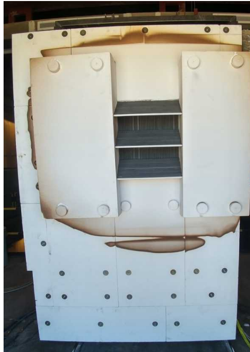
Spillage board and insulation of the receiver mounted on the structure
