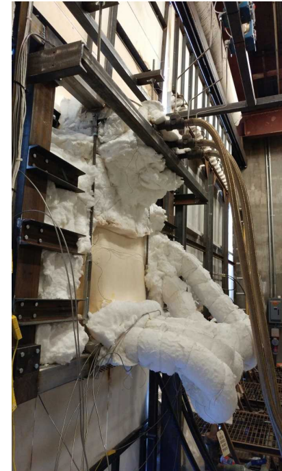
Spillage board and insulation of the receiver mounted on the structure
