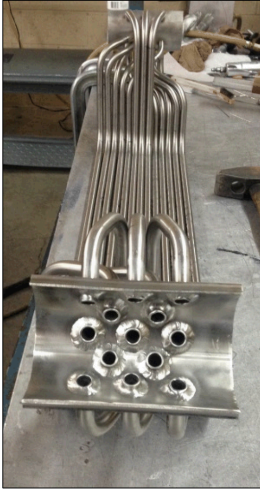
Internal welds of tubes
