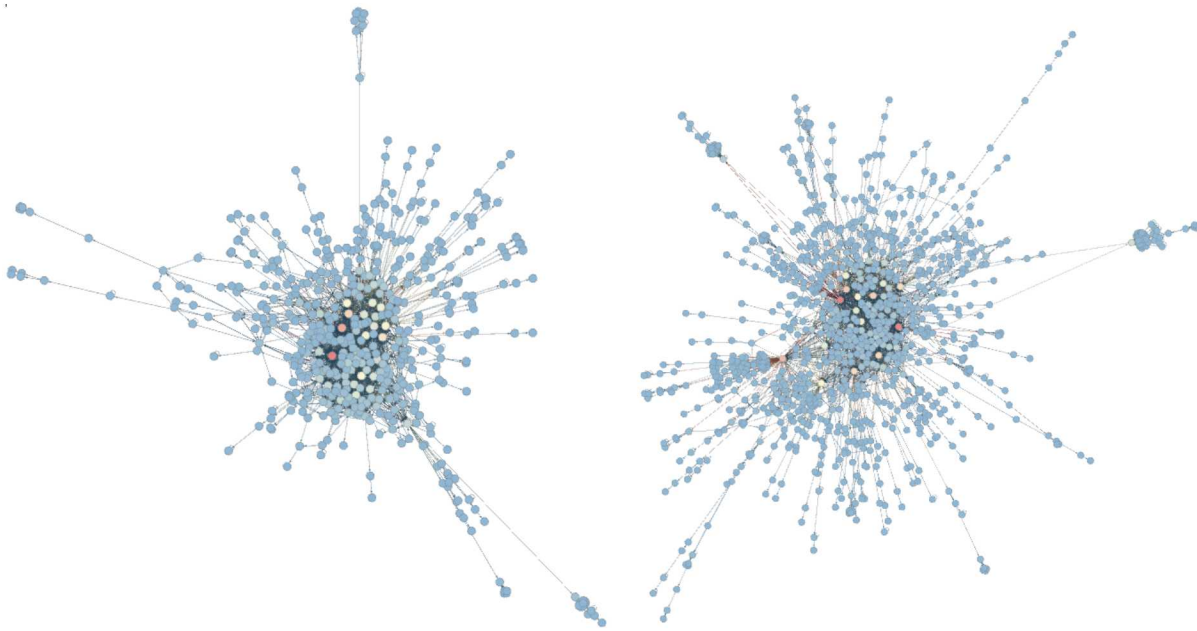
Figure 30 Two sample BGP graphs. The graph on the left has approximately 510 vertices, and the one on the right has approximately 1,100 vertices. Notice that these graphs both have a dense central cluster and chains of vertices extending off.
