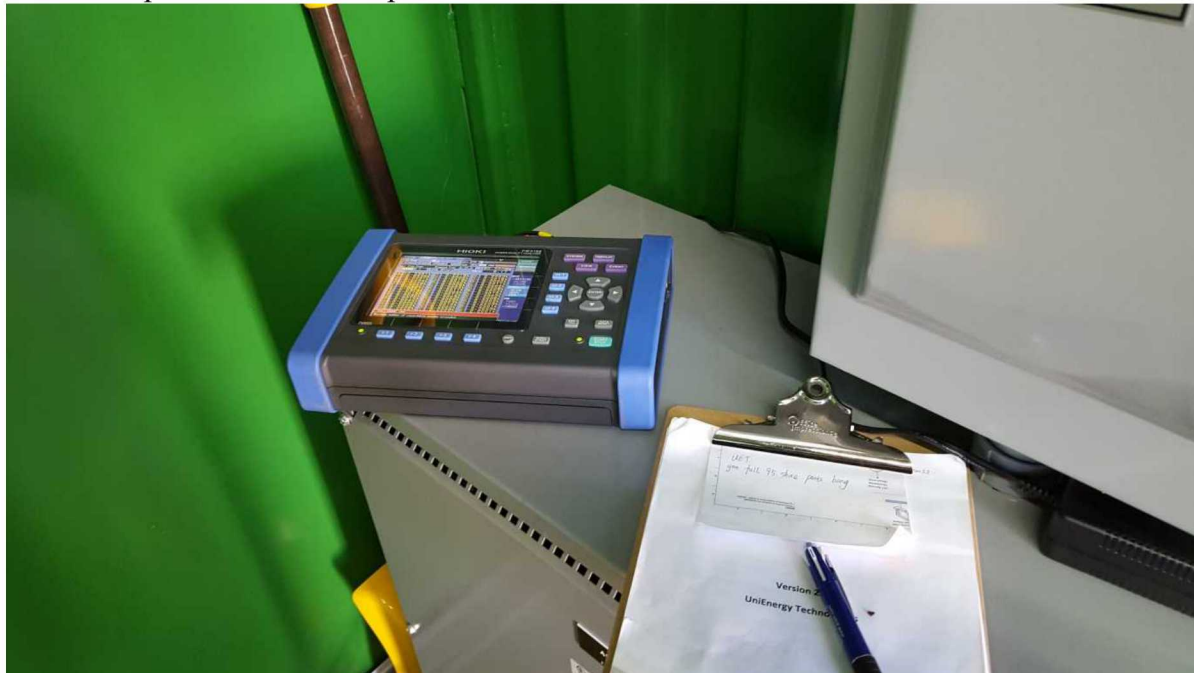
Figure 4 - Hioki 9624-50 meter installed at one Uni.System™ battery string
