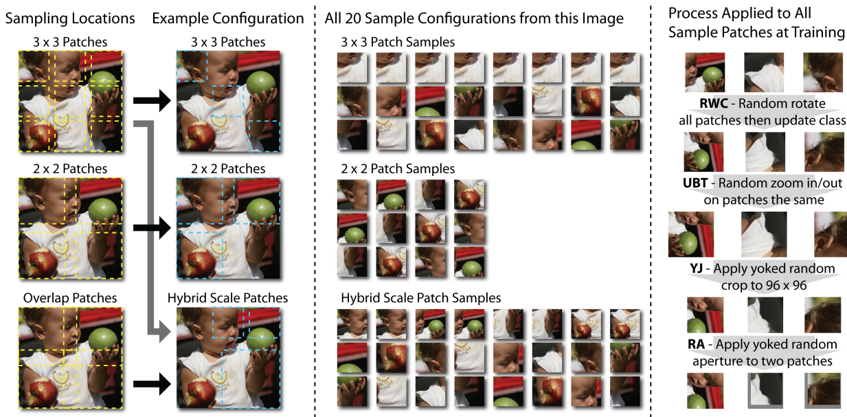
Figure 2. The left column shows the location patches are extracted from in the image. The next column over shows some example configurations obtained from those patches. In the middle are all 20 patches extracted from this (and every) image. The right column shows how these patches are fed into the process to then create the final patches fed into the neural network.
